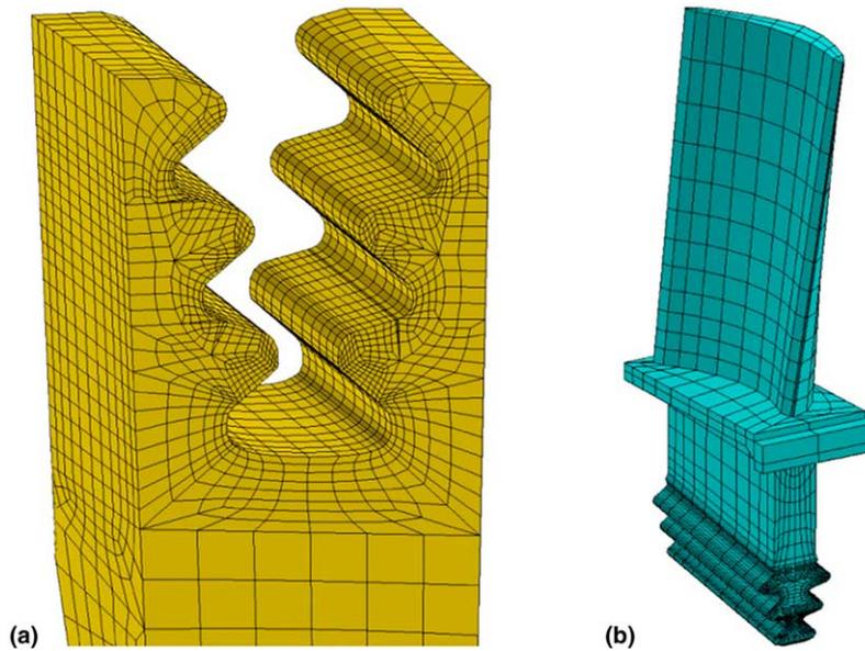
Fig. 4. Finite element models of the disc segment (a) and blade (b).
