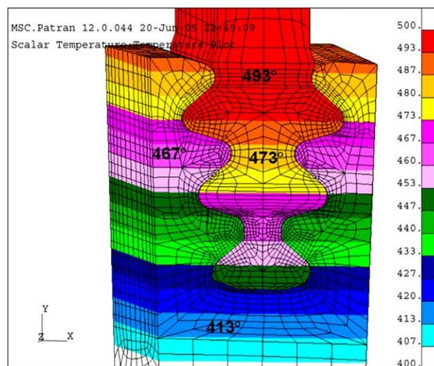
Fig. 6. Thermal field defined for models of disc and blade in the dovetail-rim region (Celsius scale).
