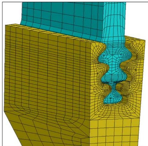
Fig. 5. Assembled model of the disc/blade segment in the vicinity of fir-tree slots.
