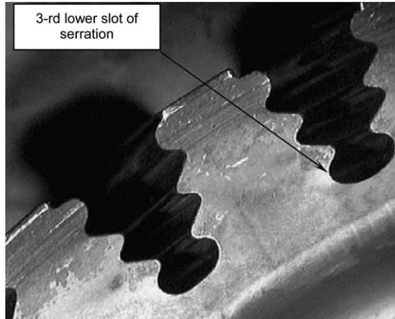
Fig. 1. The dovetail-rim area (fir-tree slots, serration fitting) of turbine disc.
