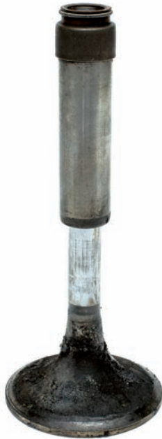
Fig. 1a Valve with seizure in the guide
