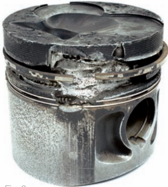
Fig. 2 Ring belt with shiny surface
