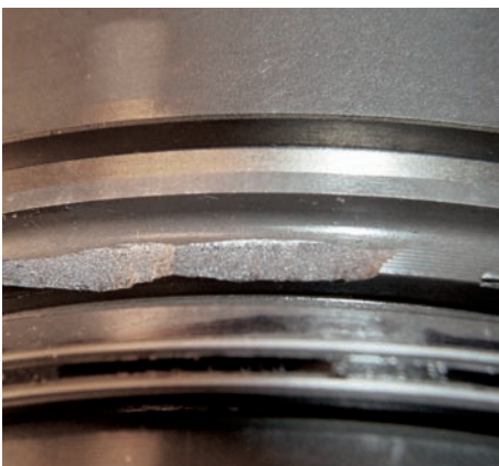
Fig. 2 Broken piston ring lands caused by an assembly error
