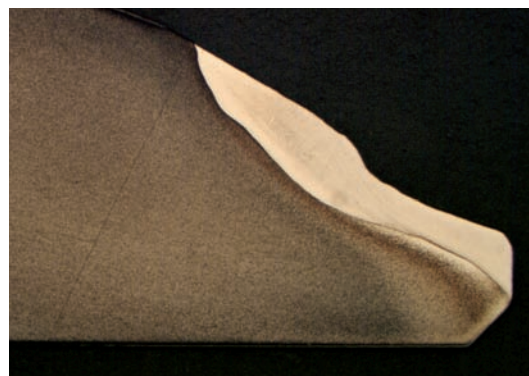
Fig. 3 Heavily worn sealing surface (stellite hardened)
