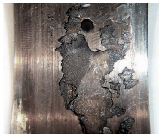
Fig. 1b Close-up view of the damaged bearing layer
