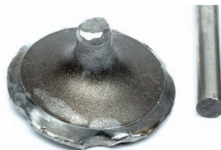
Fig. 2 Snapped off valve head
