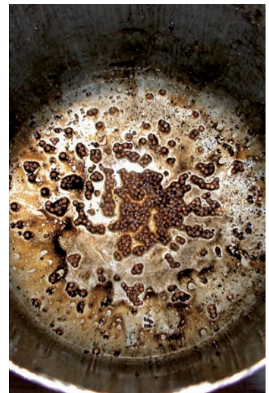
Fig. 3 Granules, water and oil in the air dryer cartridge
