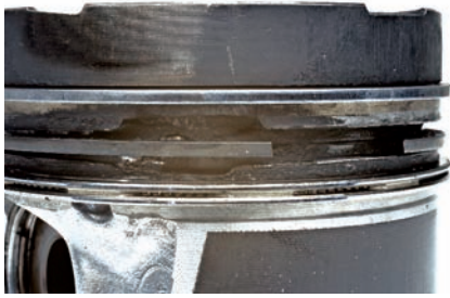
Fig. 1 Heavily worn piston ring groove
