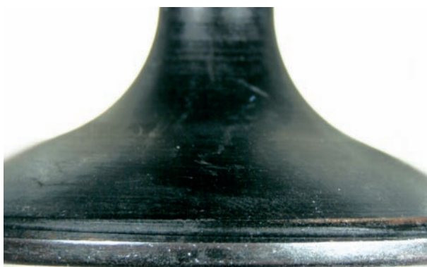
Fig. 1 Deformed valve head (tulip-shaped)
