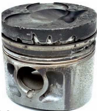
Fig. 3 Damage to the top of the piston due to individual fragments of the ring insert
