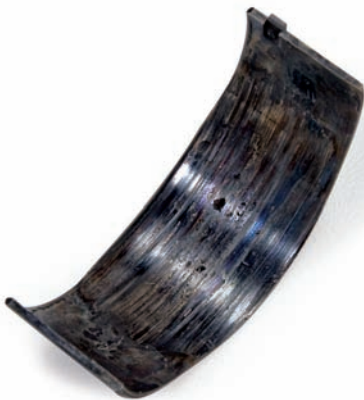
Fig. 2 Heavily worn and spun bearing
