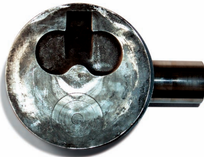
Fig. 1 Top of the piston with valve impact
