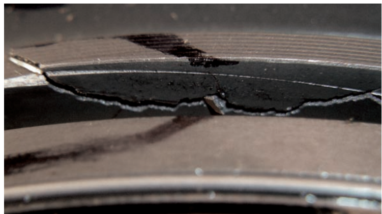
Fig. 3 Assembly error with an imprint of the piston ring
