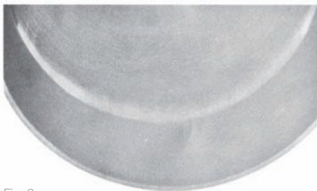
Fig. 2 Continuous, shiny line at the cylinder bore
