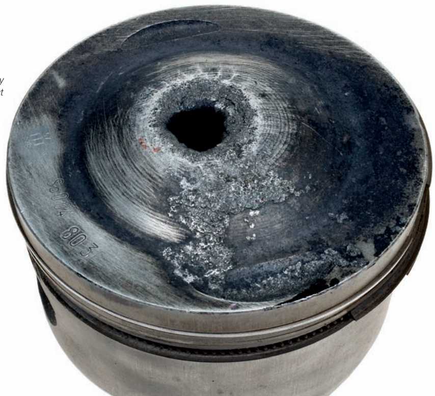
Fig. 1 Hole in the top of the piston, caused by the use of spark plugs with an incorrect heat value
