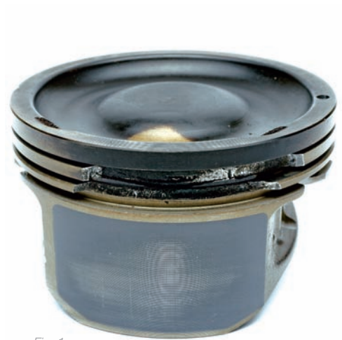
Fig. 1a Broken piston ring lands caused by an abnormal combustion
