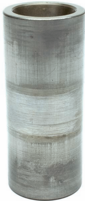
Fig. 6 Worn piston pin
