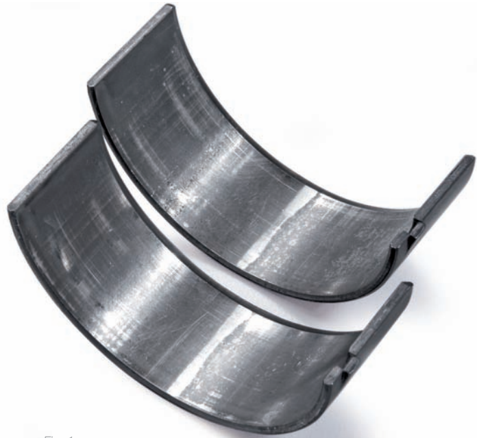
Fig. 1 Worn outer edges of a bearing
