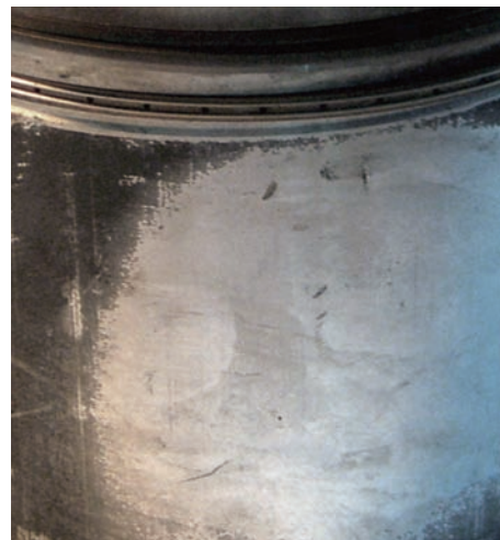
Fig. 1 Wide wear pattern and scoring marks due to fuel dilution
