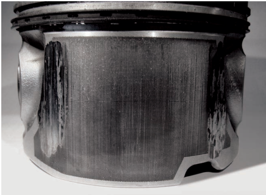
Fig. 2 Lateral piston seizure next to the pin bore
