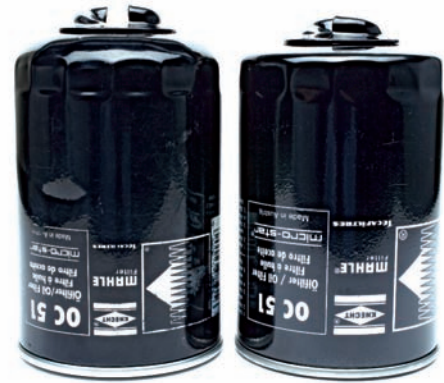
Fig. 2 For comparison: Swollen filter (left) and new filter (right)
