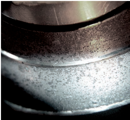
Fig.4b Even more visible when magnified: the pitting
