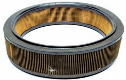
Fig. 3a Extremely dirty air filter element, filter change imperative
