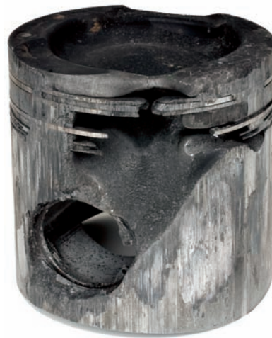
Fig. 3 Hole burned through a diesel piston
