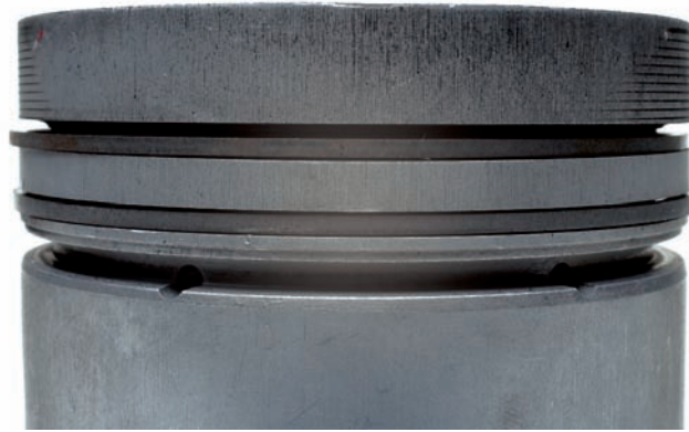
Fig. 4 Axial wear at the piston rings
