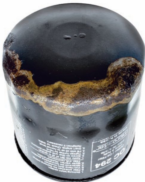
Fig. 4 Damaged coating – the result: Corrosion
