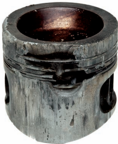
Fig. 2 Melted top land of a gasoline piston
