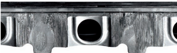
Fig. 1 Seizure at the piston skirt, caused by insufficient clearance
