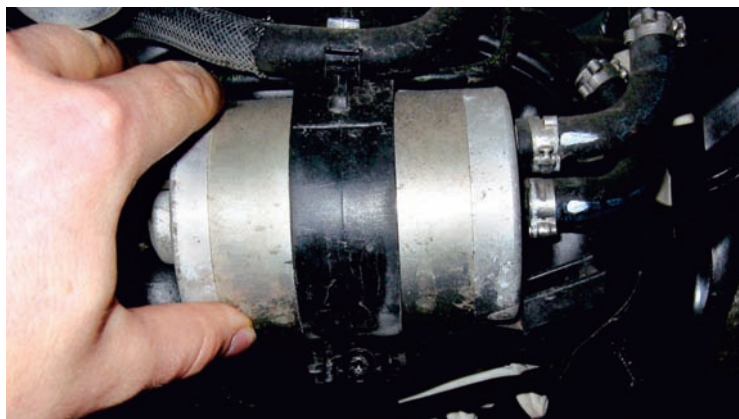
Fig. 6 Contact corrosion due to damaged insulation
