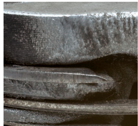
Fig. 1 Erosion at a gasoline piston
