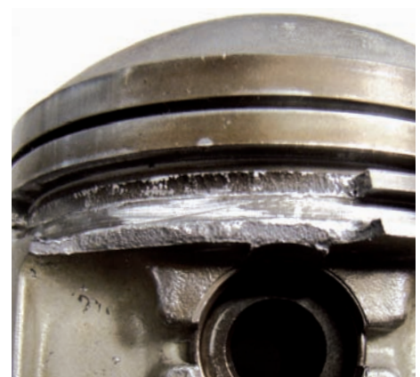
Fig. 1b Close-up view of the fracture behaviour from top to bottom
