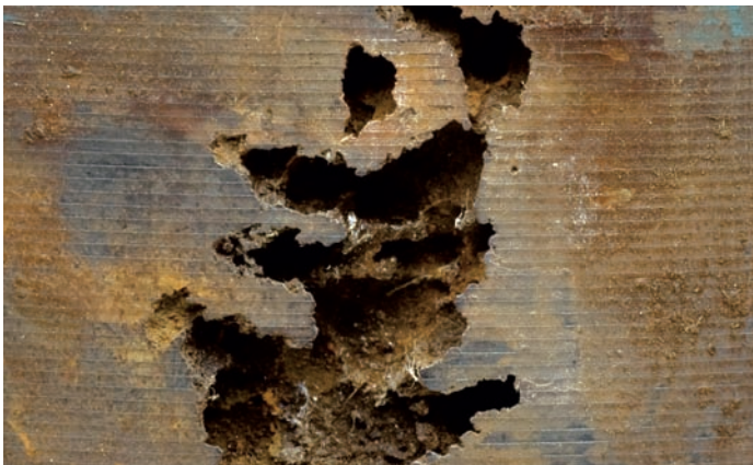
Fig. 1b Close-up view of the cylinder liner with sharp edges and cavities which become larger towards the inside
