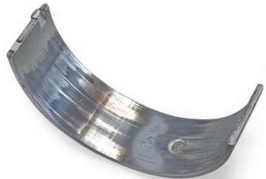
Fig. 2 Uneven wear at the bearings
