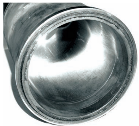
Fig. 3 Worn cylinder liner
