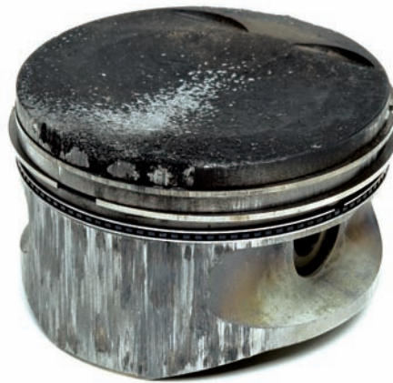
Fig. 3 Heavy erosion and melting at the piston crown
