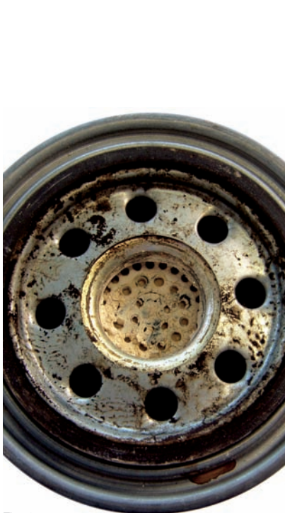
Fig. 1 Granules escaping from the air dryer cartridge
