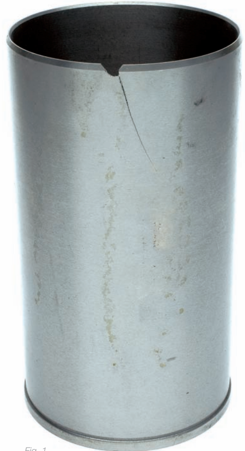
Fig. 1 Lower end of the cylinder liner with a longitudinal crack
