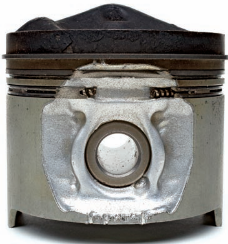
Fig. 1a Cratered piston wall, caused by a loose piston pin circlip or contamination in the piston pin
