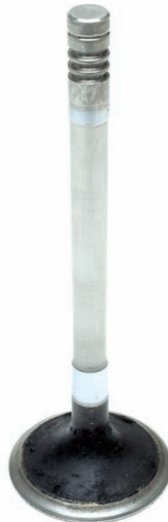
Fig. 7 Heavily worn valve stem
