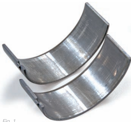
Fig. 1 Shiny marks on the running surfaces of the bearings
