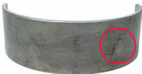
Fig. 4 Incorrectly installed bearing – at the outer surface: Imprints of the oil feeder holes
