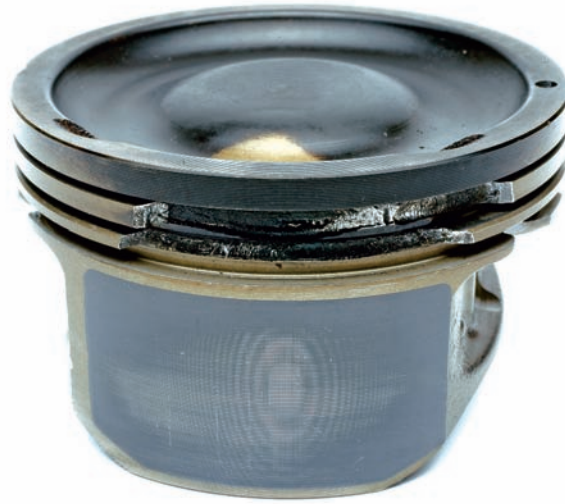
Fig. 2a Broken piston ring lands
