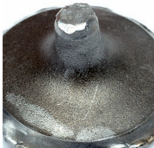
Fig. 3 Vibration fracture with fracture surface at the valve stem
