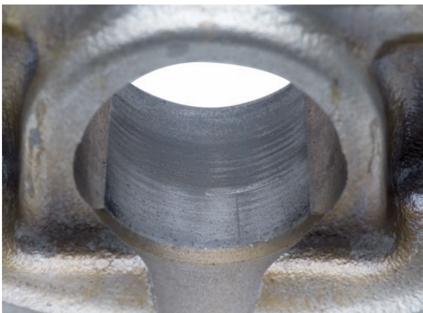
Fig. 3 Pin bore with seizure marks
