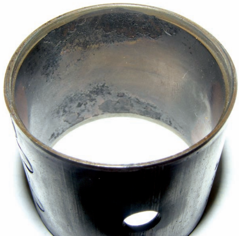
Fig. 2 Damaged connecting rod bushing
