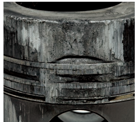
Fig. 1 Melting at the top land of a diesel piston
