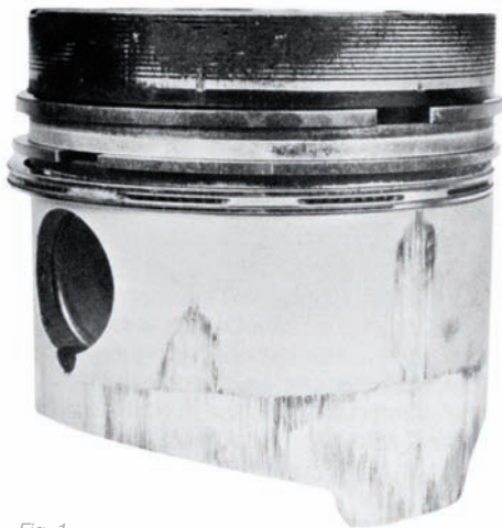
Fig. 1 Seizure at the lower piston skirt due to constriction of the cylinder liner
