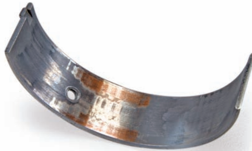
Fig. 1 Uneven wear at the bearings, the bearing layer has been partially removed
