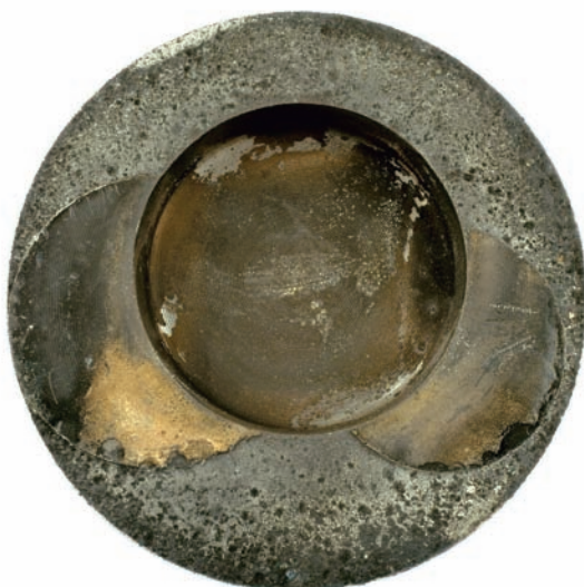
Fig. 2 Piston which has had contact with the cylinder head
