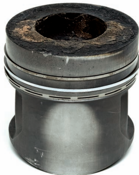
Fig. 1 Wear caused by contamination at the piston skirt
