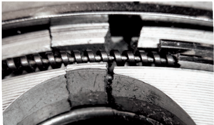
Fig. 3b Close-up view of an overload fracture
