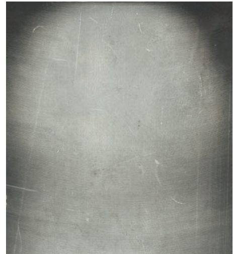
Fig. 2 Partially removed machining profile at the piston skirt
