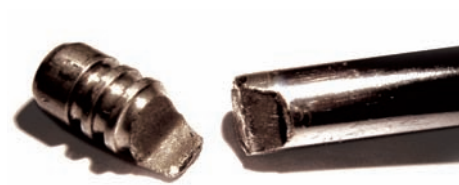
Fig. 2 Valve base broken in the groove (overload fracture/bending stress)
