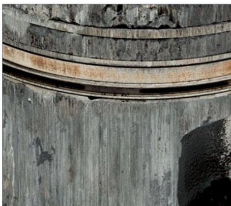
Fig. 2 Piston rings with burn marks
