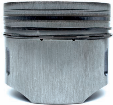
Fig. 1 Wear caused by contamination at the piston – longitudinal scoring marks
