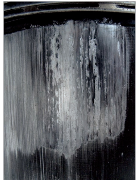
Fig. 2 Partially shiny seizure marks
