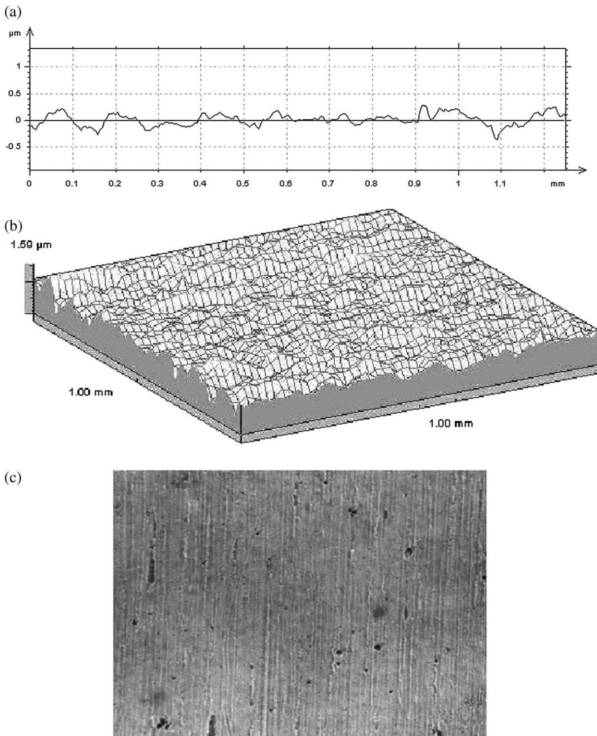
**Fig. 3.** Polished coating: a) profilogram, b) 3D scan, c) view (mag. ~110×).
