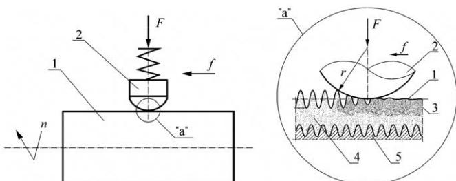
**Fig. 1.** Scheme of slide diamond burnishing: 1—workpiece, 2—burnishing tool, 3—zone of plastic deformation, 4—chromium coating, 5—steel base,  $F$ —burnishing force,  $f$ —feed,  $n$ —workpiece rotation,  $r$ —radius of tool tip.
