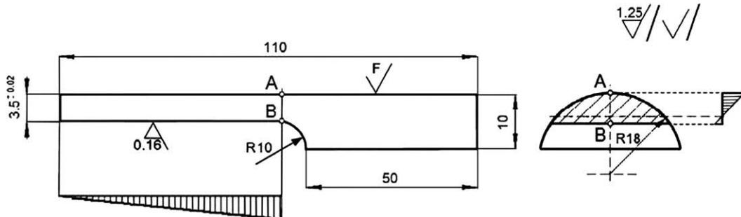
Fig. 2. Fatigue test sample geometry and theoretical stress distribution: F—surface roughness R<sub>a</sub> after final technological operation.
