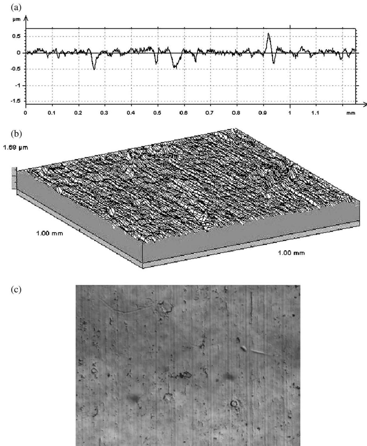
**Fig. 4.** Slide burnished coating: a) profilogram, b) 3D scan, c) view (mag. ~110×).
