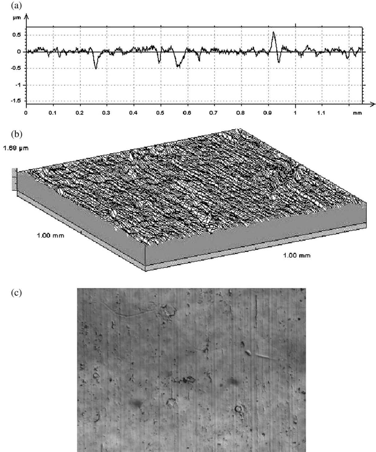
Fig. 4. Slide burnished coating: a) profilogram, b) 3D scan, c) view (mag.  $\sim 110\times$ ).
