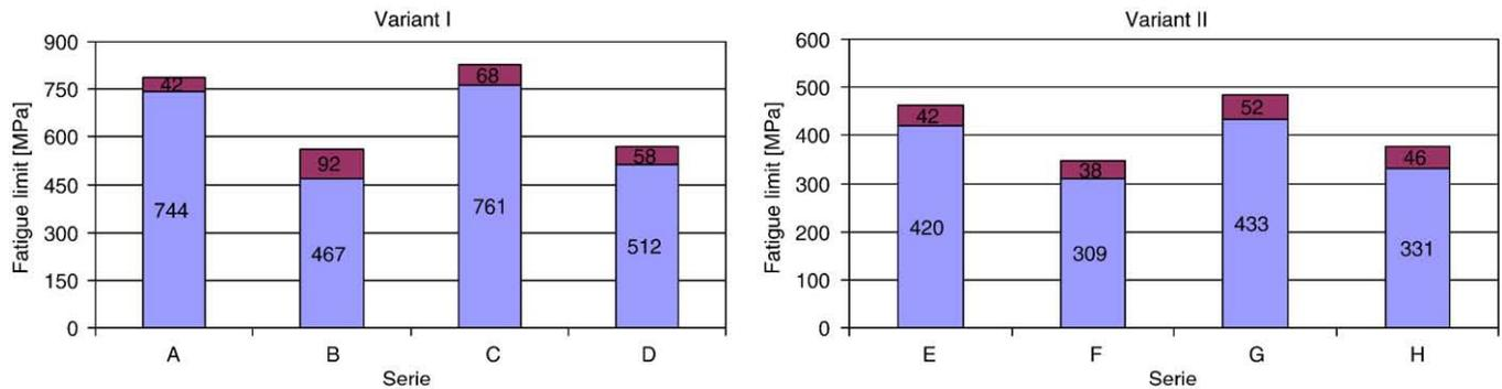
Fig. 6. Fatigue strength limit after various finishing methods, minimum levels were written and confidence intervals calculated at 5% significance level (denotations according to Table 2).
