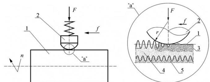
Fig. 1. Scheme of slide diamond burnishing: 1–workpiece, 2–burnishing tool, 3–zone of plastic deformation, 4–chromium coating, 5–steel base,  $F$ –burnishing force,  $f$ –feed,  $n$ –workpiece rotation,  $r$ –radius of tool tip.
