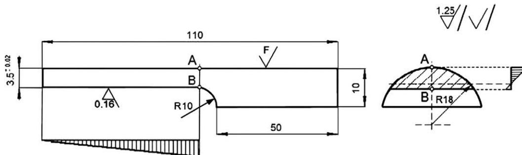
Fig. 2. Fatigue test sample geometry and theoretical stress distribution: F—surface roughness  $Ra$  after final technological operation.
