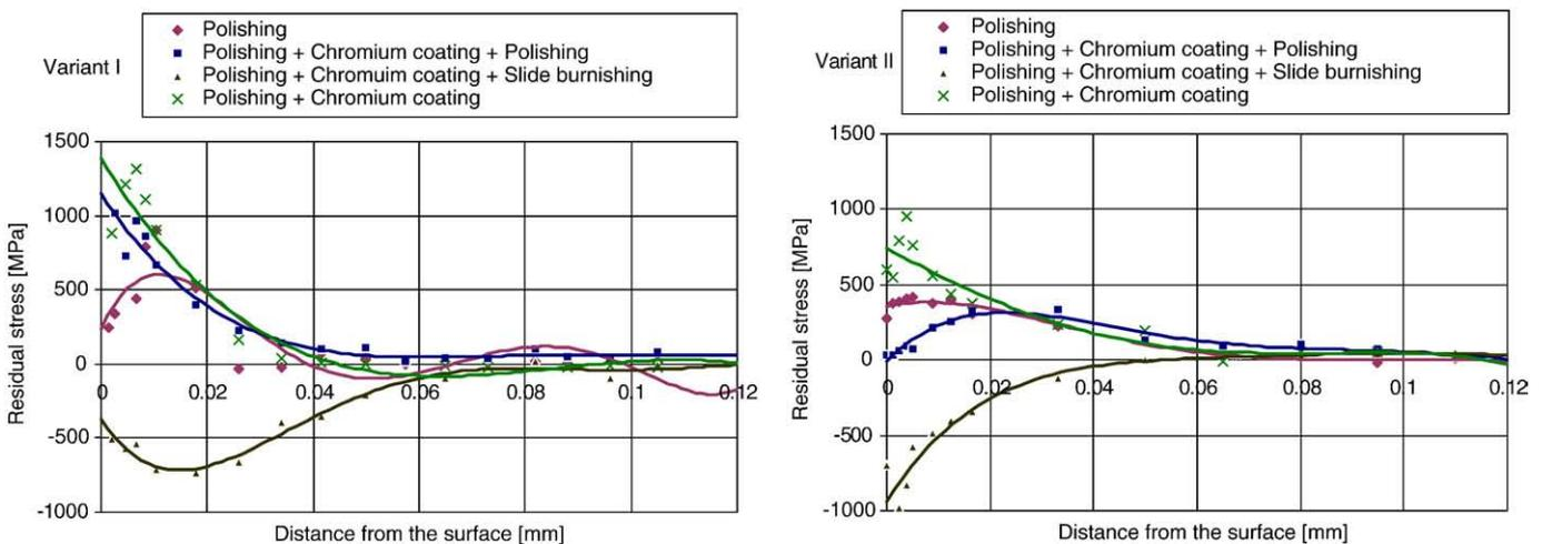
Fig. 5. Longitudinal residual stress distribution in surface layer.
