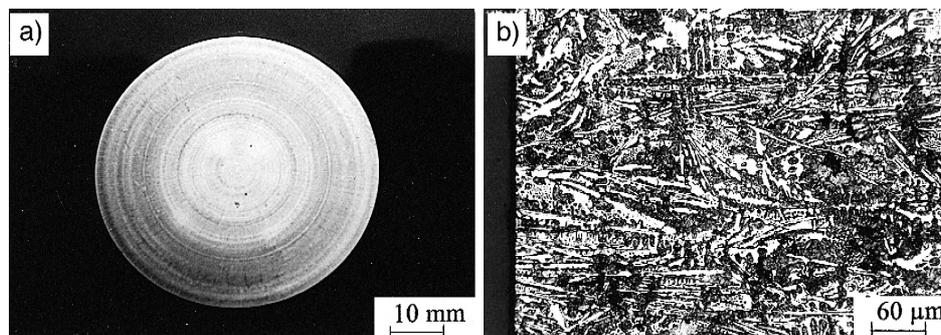
Fig. 3. Follower F1. Macrograph of the face surface (a), microstructure of the surface layer-transformed ledeburite (b).
