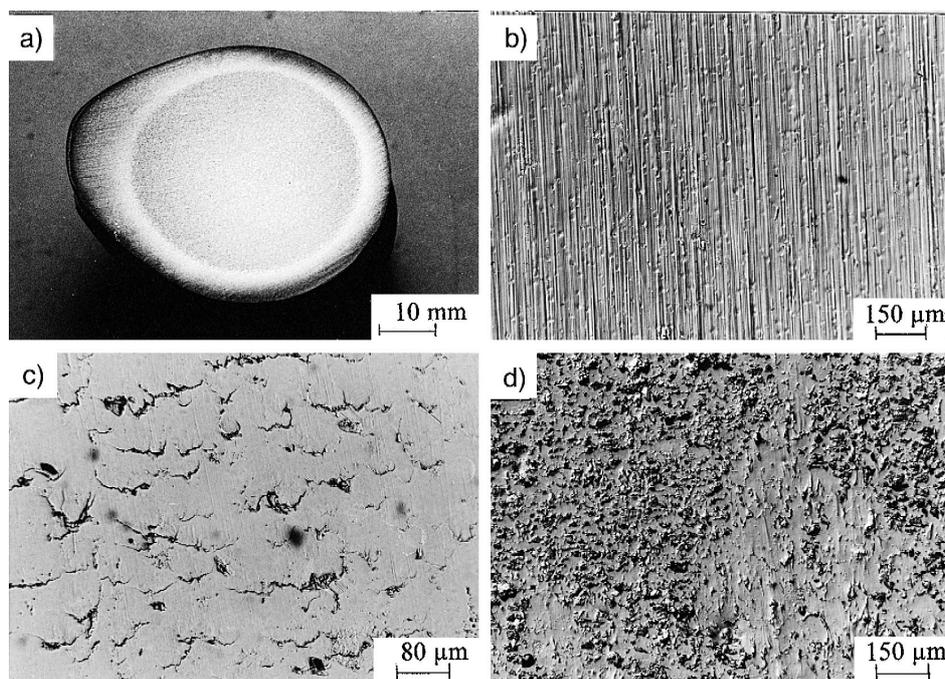
Fig. 4. Cam C2. Crosssection with a dark layer hardened on the circumference (a), the surface of a grinding cam (b), numerous cracks in the cam flank perpendicular to the direction of the slide on the follower face (c), numerous scaling cavities in the metal near the lobe of the cam (d).
