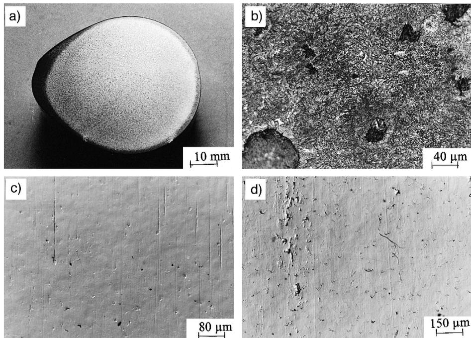
Fig. 8. Cam C1. Crosssection with a dark hardened layer on the circumference (a), hardened layer-nodular graphite, fine-acicular martensite (b), the surface of a cam flank with smooth abrasive wear (c), a strip of chippings and surface originated cracking on the shaft (d).
