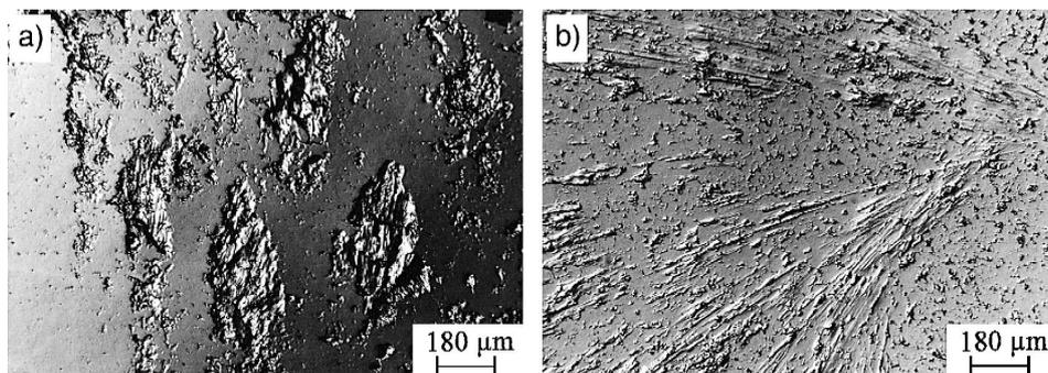
Fig. 10. Surfaces of cam 7 and follower F4. The lobe of the cam with metal fragments torn off the surface layer and chipped cementite particles (a), follower with cementite chippings and traces of surface deformation by hard particles (b).
