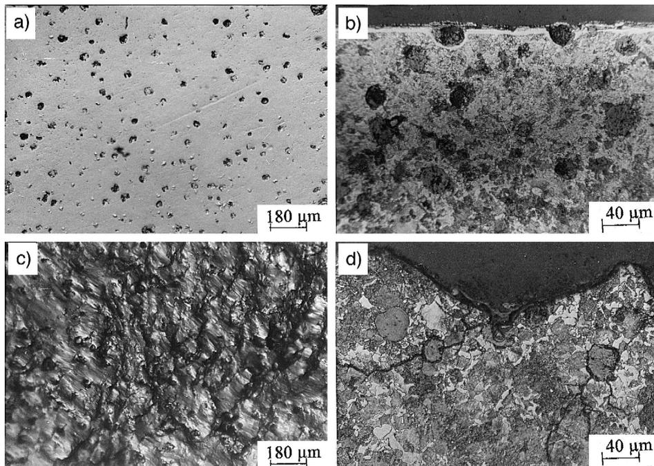
Fig. 6. Cams C4 and C5. Smooth worn surface of shaft C5 after  $0.8 \cdot 10^6$  revolutions (a), ion nitrided diffusion layer of shaft C5 together with pearlite, ferrite and nodular graphite structures after  $0.8 \cdot 10^6$  revolutions (b), scaled C4 shaft surface after sulfonitriding together with pearlite, ferrite and nodular graphite structures (c), down-to-the base cracks propagating from the scaled C4 shaft surface after sulfonitriding (d).
