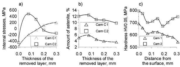
Fig. 7. Change in internal stress (a), participation of retained austenite (b), microhardness (c) in the function of the distance from the surfaces of cams C1 and C2.
