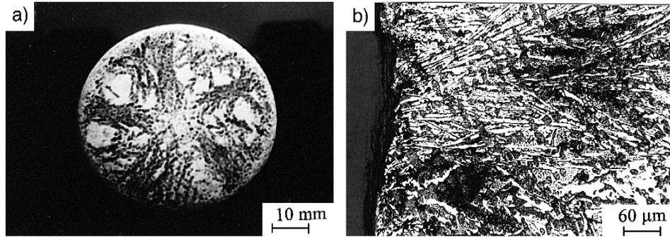
Fig. 5. Follower F2. Macrophotography of the face surface (a), microstructure of the surface layer-transformed ledeburite, separated metal fragments, broken cementite plates (b).
