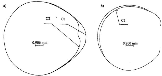
Fig. 9. Outlines of worn out C1 and C2 cams (a), outlines of a fragment of a worn out C2 cam with its outline before the lift test (b).
